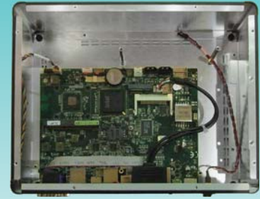
MiTex-P Chassis without top-cover
